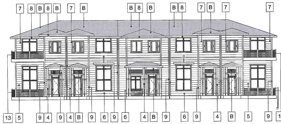
③ Building A, 5 Plex, South Elevation, Materials 1/8" = 1'-0"
