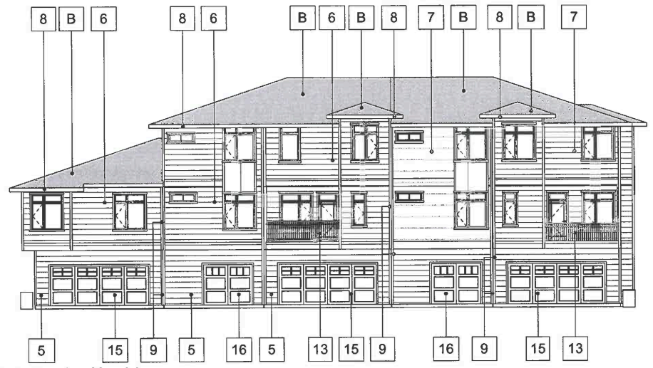
① Building E, 5 Plex, North Elevation, Materials 1/8" = 1'-0"
