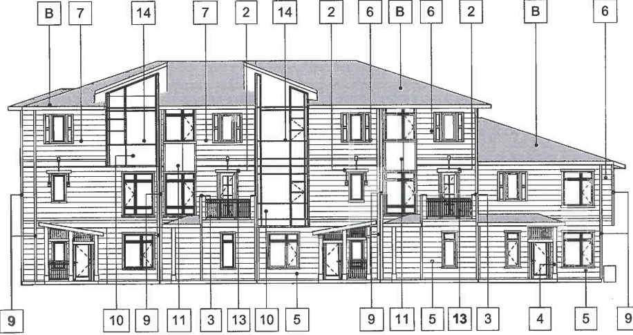
③ Building E, 5 Plex, South Elevation, Materials 1/8" = 1'-0"
