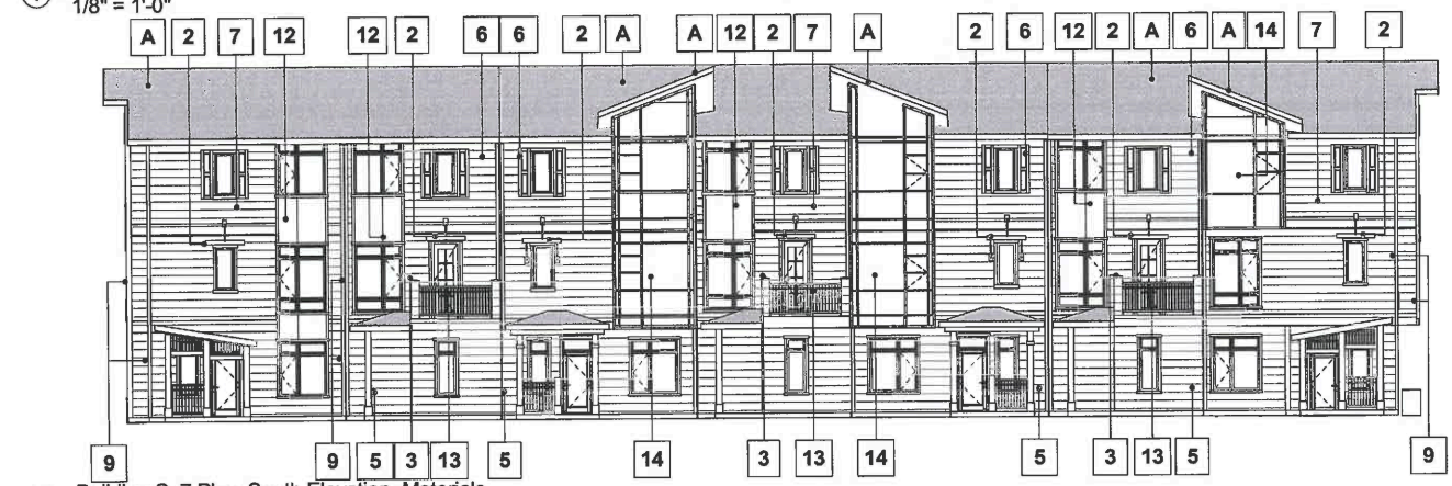
3 Building C, 7 Plex, South Elevation, Materials 1/8" = 1'-0"
