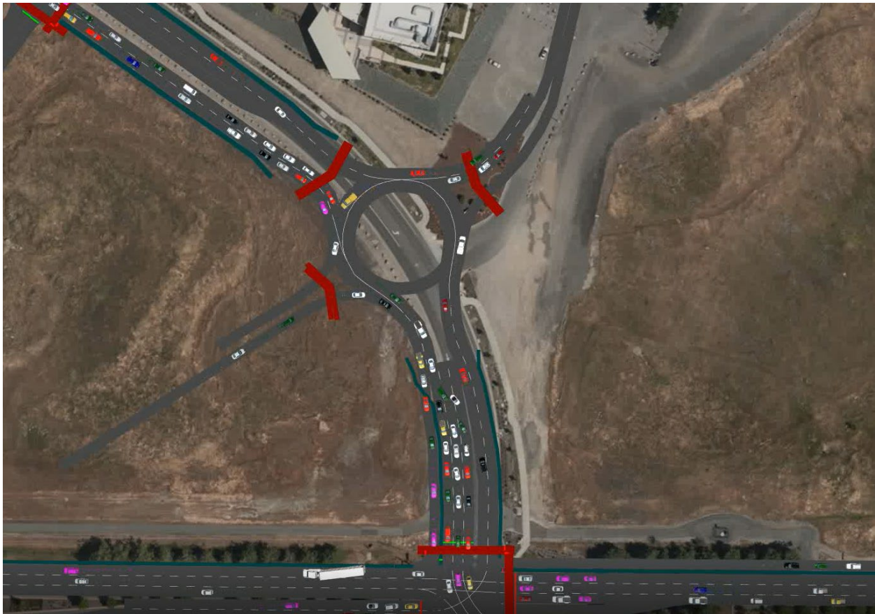
Figure 5: Vissim microsimulation model of the University Ave. corridor north of Sunset Blvd.
