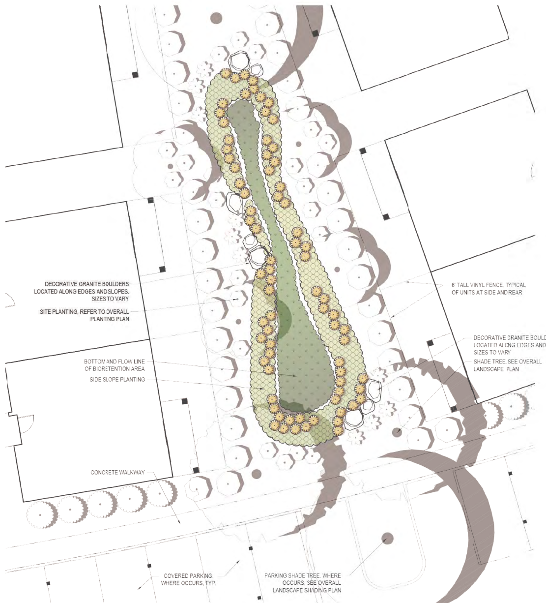
1 TYPICAL BIORETENTION PLANTING AS SHOWN
